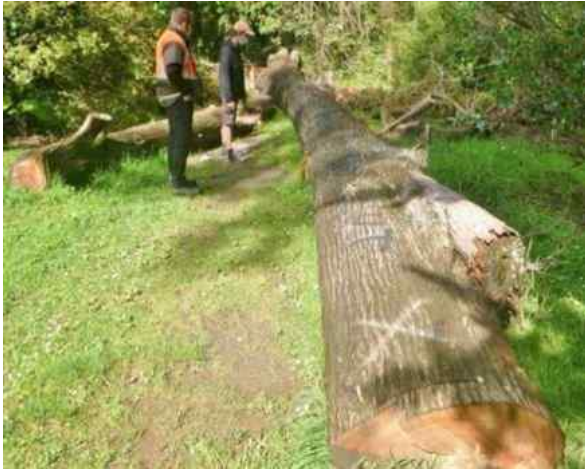
Donovan Richmond of Treescape and Tony Lyon of the TPS inspect an 18-m trunk for potential ferry timber. Unsound at the butt and solid towards the crown, it provided four 3-m logs, and fifteen short logs came from other trees.
