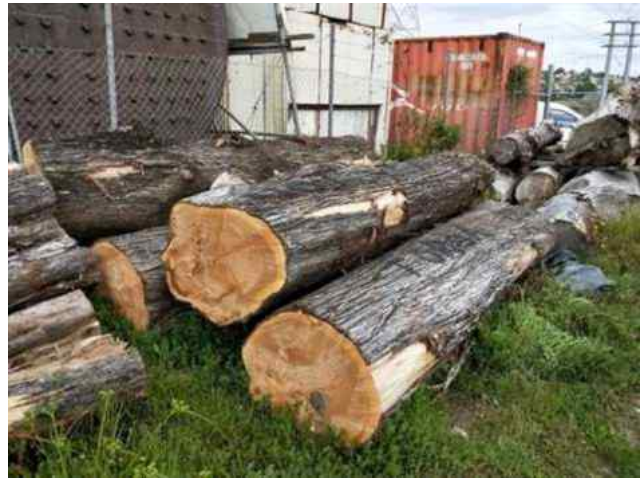
Donovan Richmond of Treescape and Tony Lyon of the TPS inspect an 18-m trunk for potential ferry timber. Unsound at the butt and solid towards the crown, it provided four 3-m logs, and fifteen short logs came from other trees.
